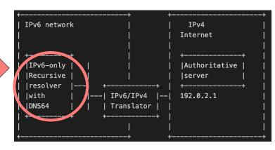
The network topology we want to achieve. The Resolver is inside the IPv6 only network.
